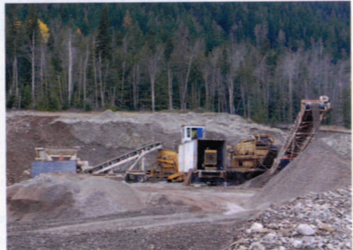
High clay and moisture content was causing screening issues for Morrissey Aggregates in Fernie, B.C. They fixed the problem with new screens. (Photo by Rebecca Edwards)
